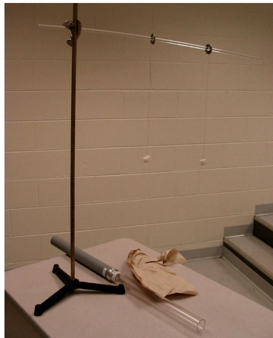
Jumbo Electrostatic and 'Pith' Ball Setup The wire leads to an insulated, conducting sphere.
